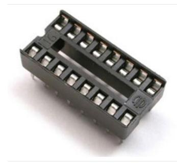
The latest kits from Adafruit come with 2 16-pin sockets for the L293D motor drivers. They are OPTIONAL and not necessary for operation.
