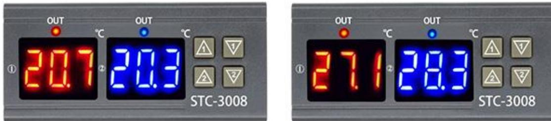
Long press  $\Delta$  3 seconds, the first group start temperature flash (default 25 ° C) press the plus or minus button to adjust, long press  $\nabla$  3 seconds, stop the temperature value flash (default 40 ° C) press the plus or minus button to adjust.
